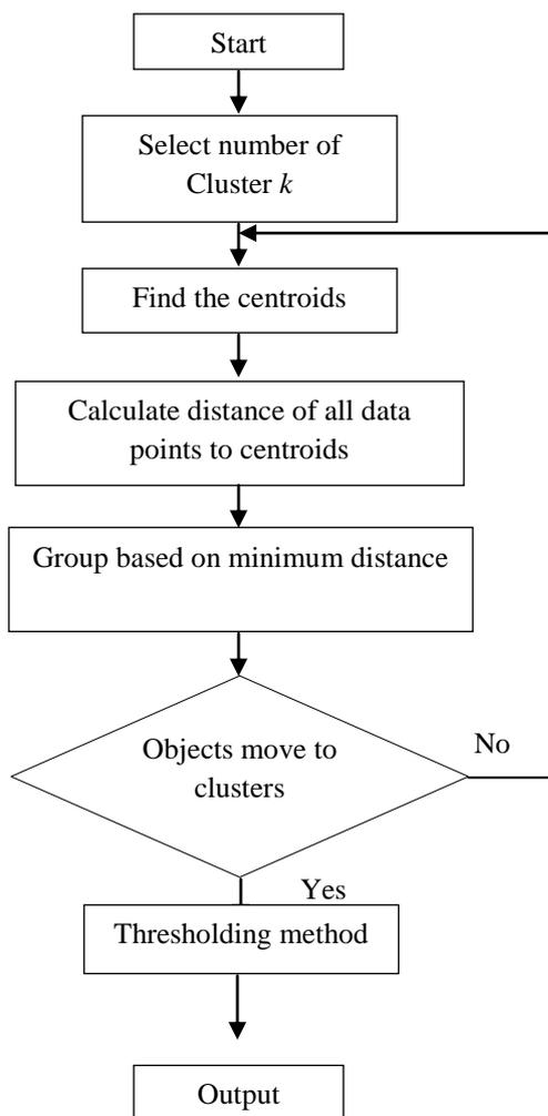
**Fig.1 Process in k-means clustering algorithm and Thresholding Method**
