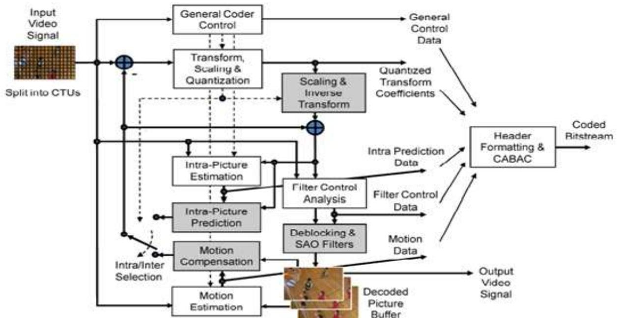
Figure 1: Block diagram of HEVC encoder.
