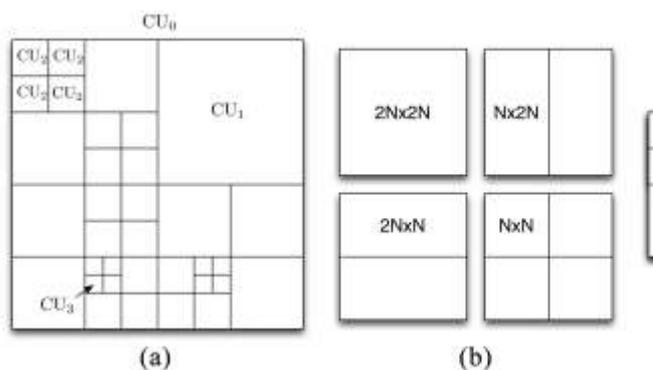
Figure 2: Illustration of recursive CU structure in HEVC
