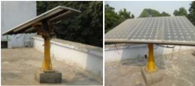
Figure 1: Developed Solar Tracing System
