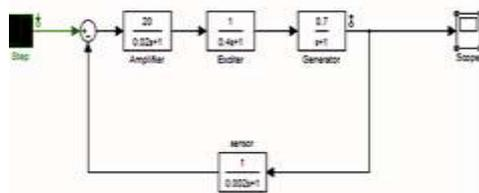
Fig.2. Simulink Model for AVR
