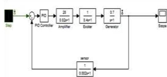
Fig.4. AVR with PID Controller
