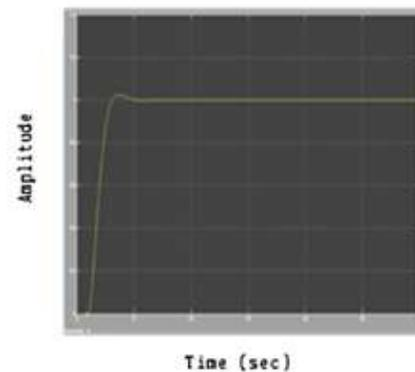
Fig.9. Output of AVR by IMC method
