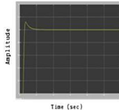
Fig.8. Output of AVR by SF method
