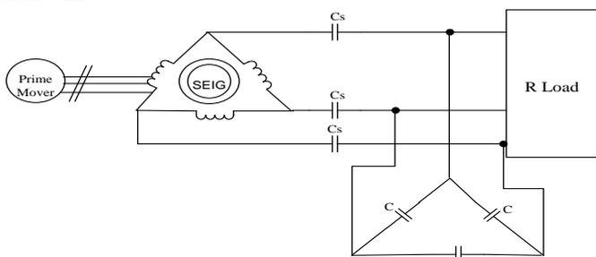
**Fig.3:** Schematic diagram of the Long-Shunt self-excited induction generator with series compensation
