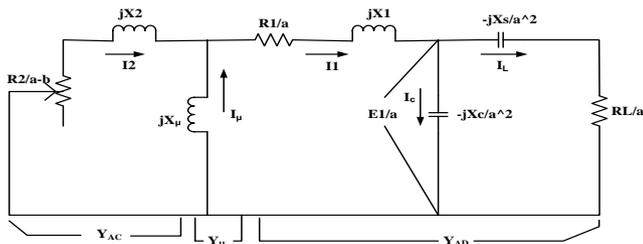
Fig 2: Steady-state equivalent circuit of the short-shunt SEIG.
