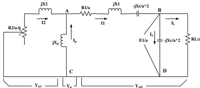
**Fig.4:** Steady-state equivalent circuit of the short-shunt SEIG.
