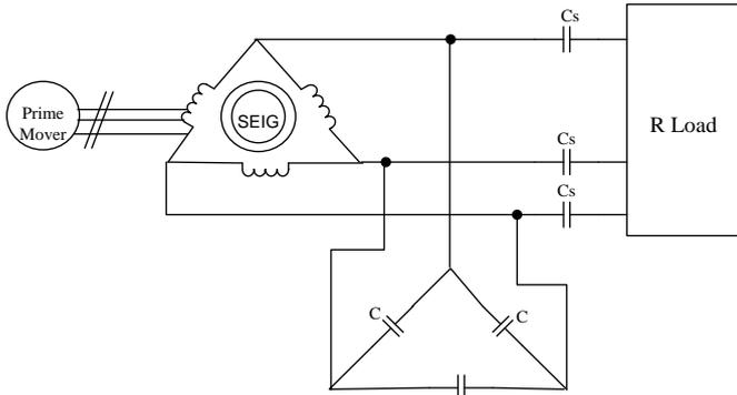
Fig 1: Schematic diagram of the Short-Shunt self-excited induction generator with series compensation.
