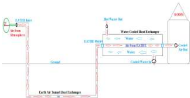
Fig. 9. Layout of EATHE Coupled with Water Cooled Heat Exchanger (Counter Flow Arrangement)
