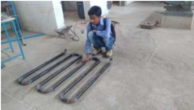
Fig. 15. Connection of Mild Steel Pipes in Series at Mechanical Workshop
