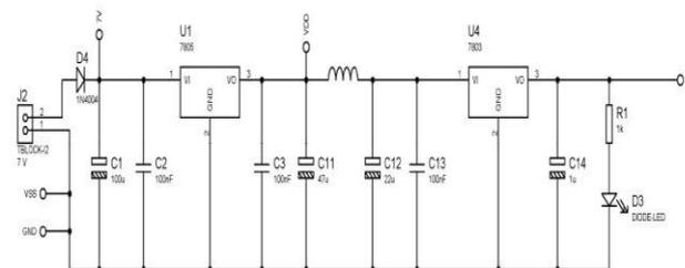
Figure 3. Diagram of the power supply
