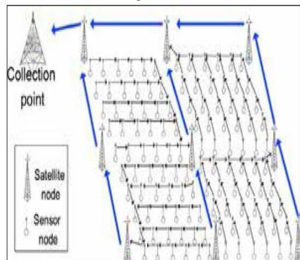
Figure 1. Network deployment in precision agriculture [8].
