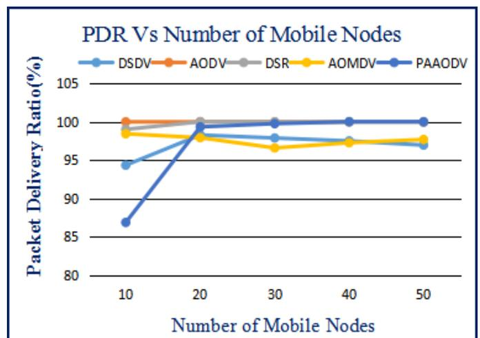
Fig.-2: Packet Delivery Ratio Vs Number of Mobile Nodes
