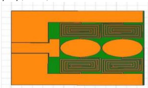
Figure 5: Geometrical model of the proposed single-band, monomode ZOR antenna (with two unit cells). [4]
