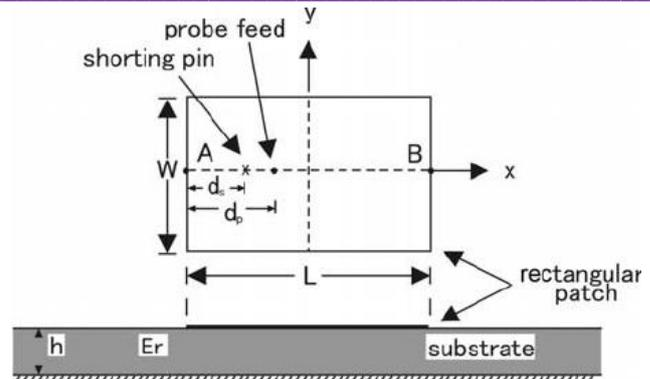
Fig 1: Configuration of microstrip antenna with shorted pinq4
