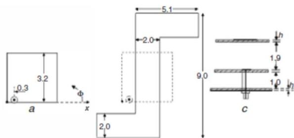
Fig 2. Design of broadband S shaped microstrip antenna
