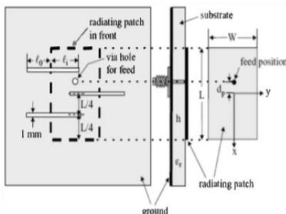
Fig 4: Design of compact microstrip antenna with meandering slots in the ground plane.
