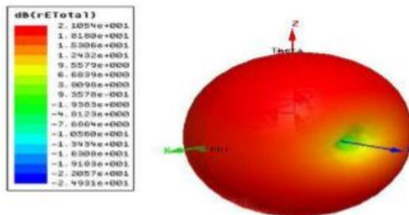
Figure 8: 3D-Gain of the proposed antenna at  $n = 0$  mode (freq = 4.88GHz) [4]
