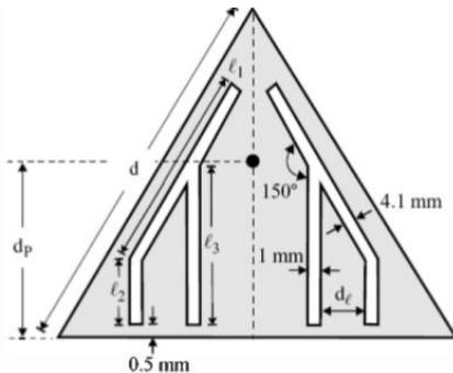
Fig 3 : Slot loaded Triangular Microstrip Patch Antenna
