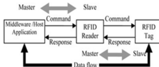
Fig.6: Working principle of RFID
