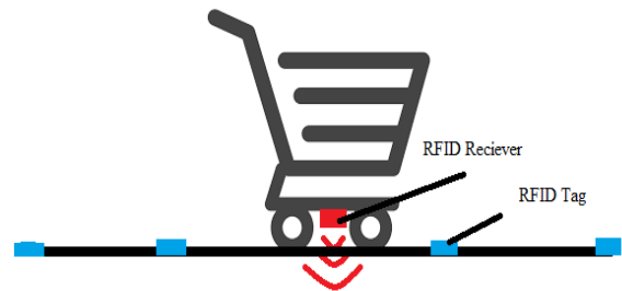
Fig.5. Illustration of RFID module installed on the cart
