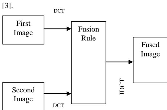
Figure1 Image Fusion with DCT [10]
