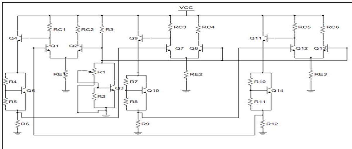
Figure 3. Circuit diagram of ECI based 3-stage Ring Oscillator. The values of circuit components: RC1 to RC6 = 1KΩ, RE1 to RE3 = 1.4KΩ, R6=R9 = R12=1KΩ. All the other resistors = 10KΩ. R1 is a variable resistor. Reference voltage is changed by varying the resistance R1. The transistors used in the circuit belong to transistor array CA3086; DC supply voltage Vcc = 5.2 volts.
