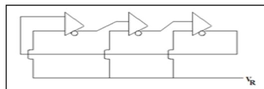
Figure 2. Functional block diagram of the 3-stage inverter based RO.
