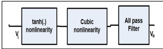
Figure 8. Proposed nonlinear model of single emitter coupled inverter stage.
