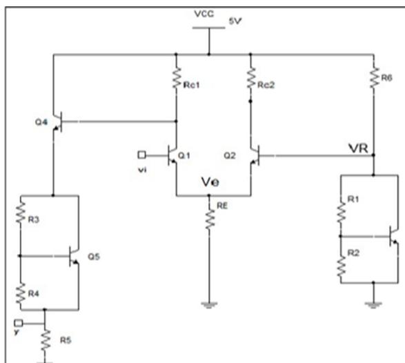
Figure 6. Experimental Circuit of Single ECL Inverter stage.
