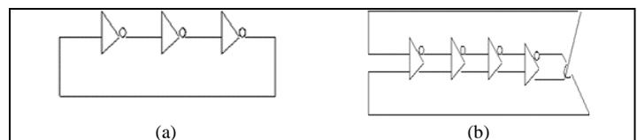
Figure 1. Ring oscillator using (a) single ended inverter, (b) differential inverter.
