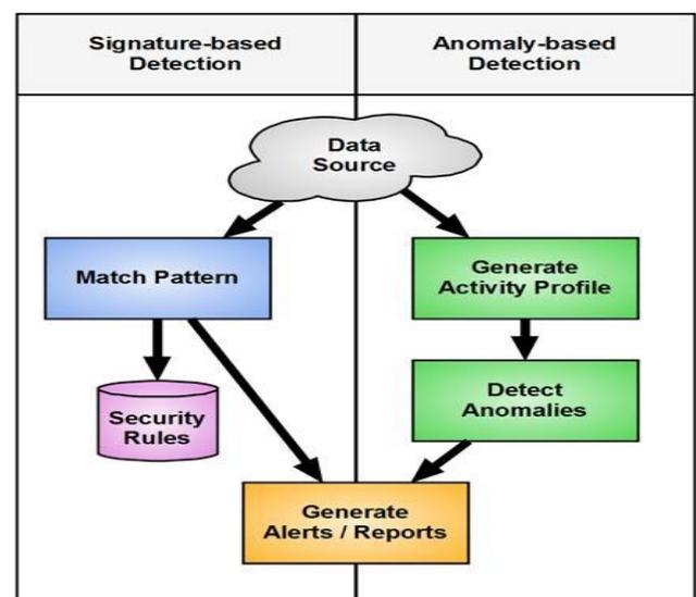
Fig.1. Flow chart of Signature and Anomaly based detection technique
