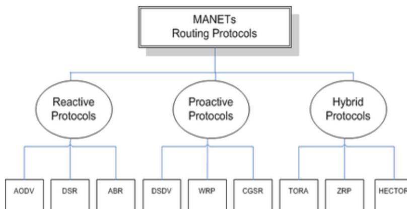
Figure 1: Proactive, Hybrid, and Reactive Routing Protocols in MANET
