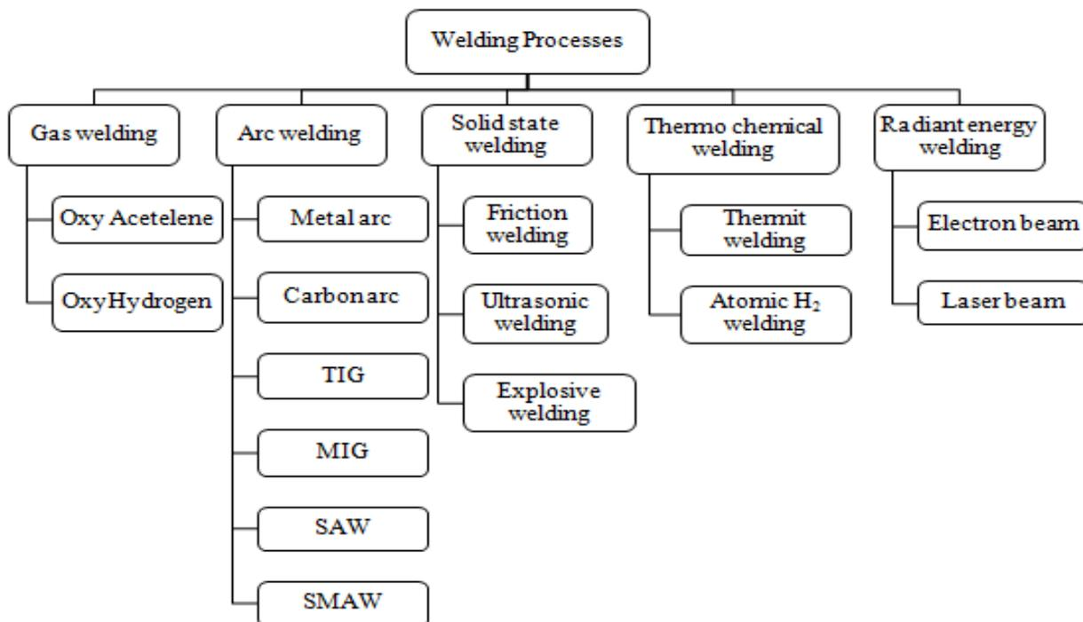
Figure 1 Classification of welding process
