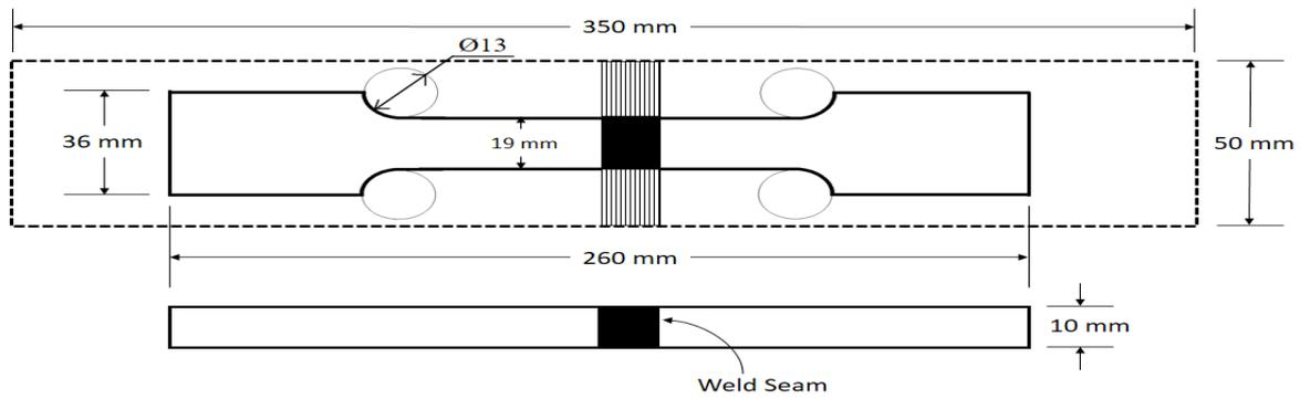
Figure 5 Tensile specimen
