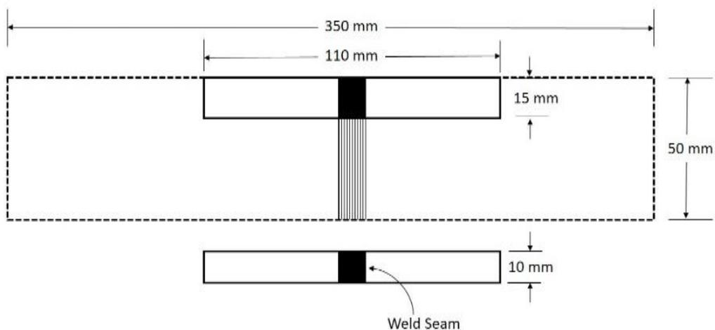
Figure 7 Hardness specimen
