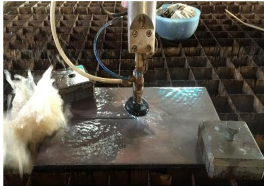
Figure 3 Water jet CNC
