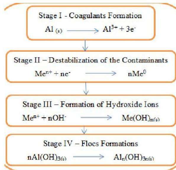
Figure 2 Stages of reactions occurring in the process
