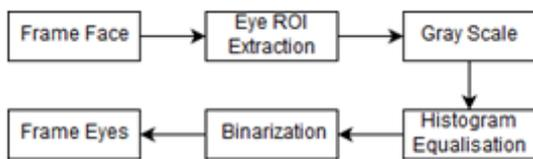
**Fig. 3 The flow diagram of eyes feature marking**
