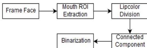
**Fig 4 The flow diagram of lips feature marked**
