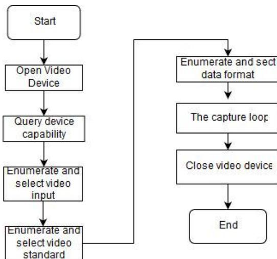
Fig. 7 The operation procedures of V4L2
