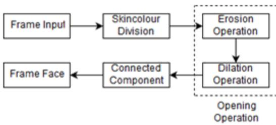
**Fig. 2 The flow diagram of face detection**
