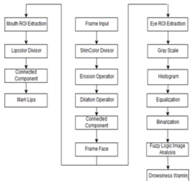
**Fig. 1 The flow diagram of fatigue recognition algorithm**
