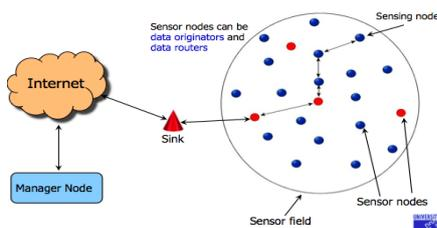
Fig 1: Structure of a WSN
