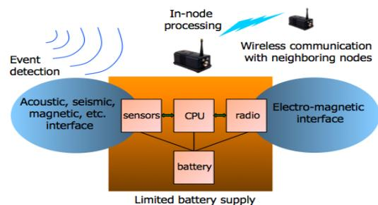
Fig 2: Blocks of Wireless Sensor Nodes
