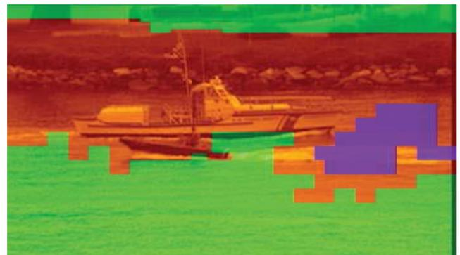
Figure 5(d): Moving region segmentation from compressed video using global motion estimation
