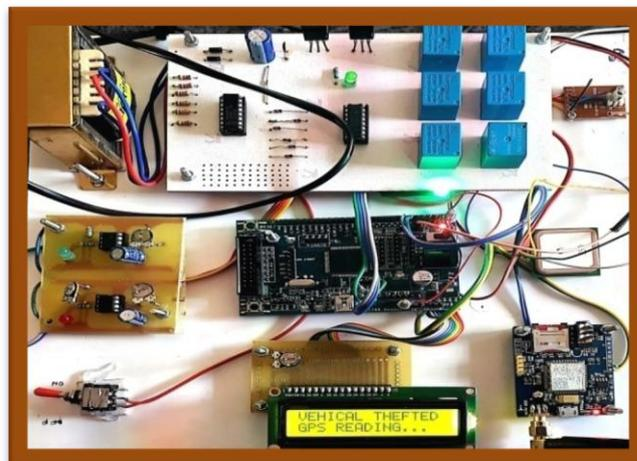
**Fig. 22:** Display of Vehicle theft detection
