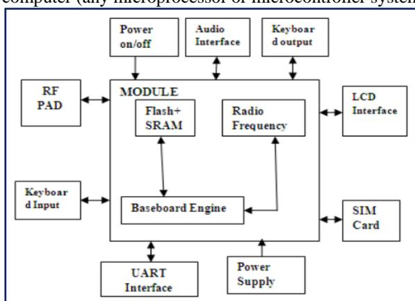
**Fig. 17:** GSM module structure
