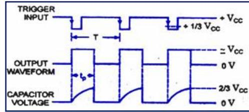
**Fig. 11:** Waveforms of Monostable multivibrator
