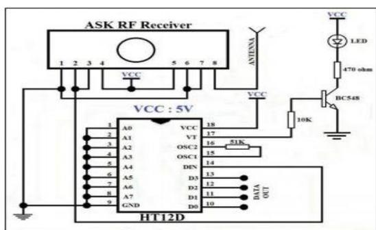
**Fig. 16:** Circuit diagram of RF receiver
