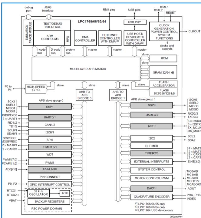
Fig. 2: Block diagram LPC 1768 ARM Cortex M-3
