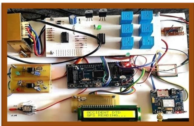
**Fig. 20:** Accident detection displays on LCD
