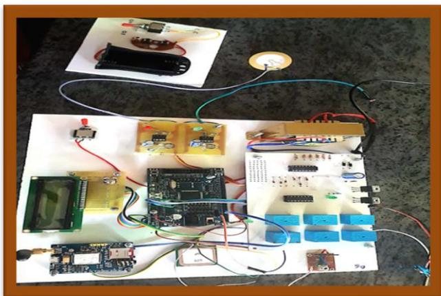
**Fig. 19:** GPS and GSM based accident location intimation, vehicle and fuel theft detection system.
