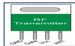
**Fig. 13:** Pin diagram of RF transmitter
