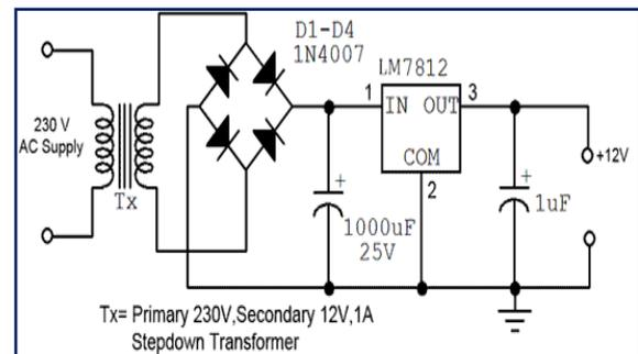
Fig. 5: Volts regulated power supply
