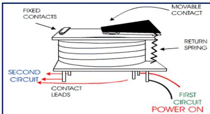
**Fig. 8:** Internal Structure of Relay
