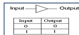
Fig. 6: Symbol and truth table of Buffer gate.
