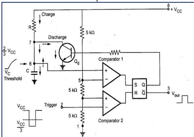
**Fig. 10:** Monostable multivibrator operation of 555 Timer.
