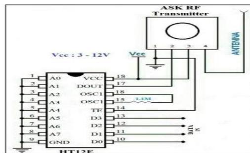
**Fig. 14:** Circuit diagram of RF transmitter
