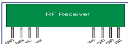
**Fig. 15:** Pin diagram of RF receiver
