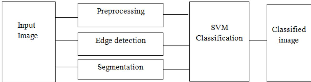
Fig 1: System Architecture
