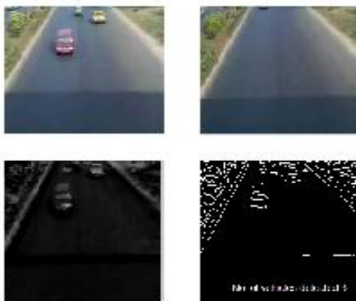
Figure 2 (a)Real-time (b)Background (c)Subtracted (d)No. of vehicles = 3
