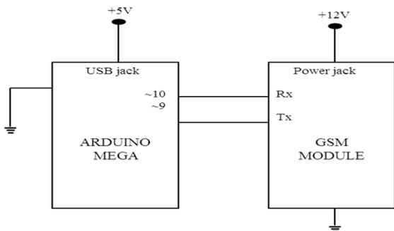
Figure 10. Interfacing of GSM module with Arduino.
