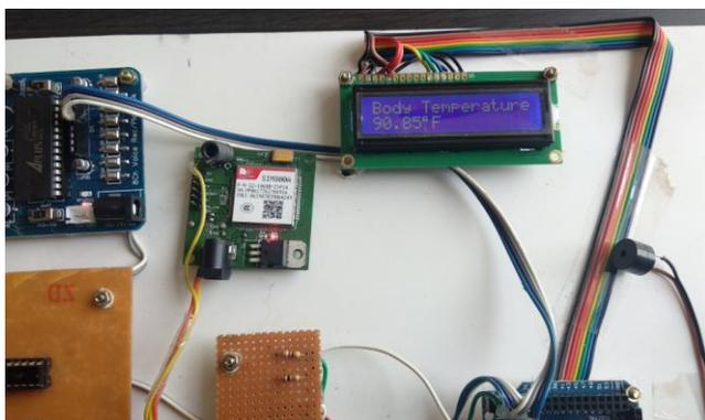
Figure 18. Displaying Body Temperature of the patient using LCD.
