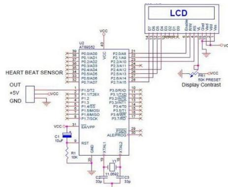
**Figure 8.** Interfacing of heart beat sensor with Arduino.
