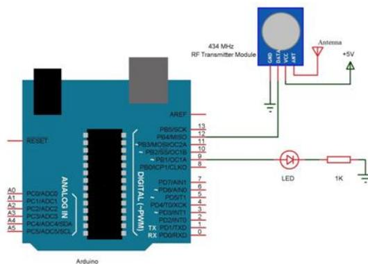
Figure 12. RF Transmitter interfacing with Arduino
