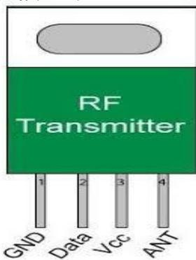
Figure 11. RF Transmitter.
