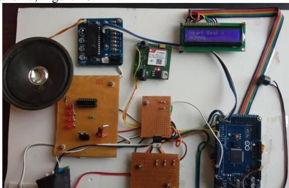
Figure 17. Displaying Heart Beat is Normal using LCD.
