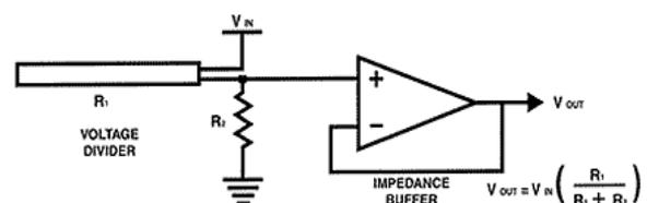
Figure 4. Flex sensor circuit.
