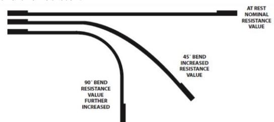
Figure 3. Change in resistance due to bend.
