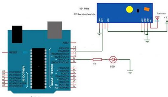
Figure 14. RF Receiver interfacing with Arduino
