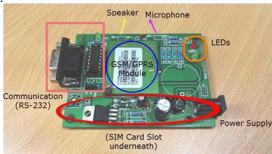
**Figure 9.** GSM SIM800
