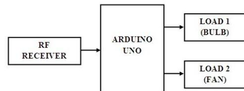
Figure 2. System architecture at control end for home automation.
