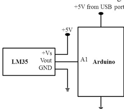
**Figure 6.** Interfacing of LM35 with Arduino.
