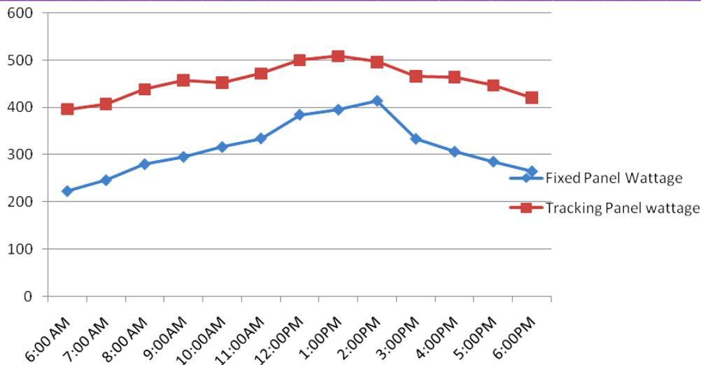
Fig. 7: Units generate graph between fixed and tracking solar Panel.
