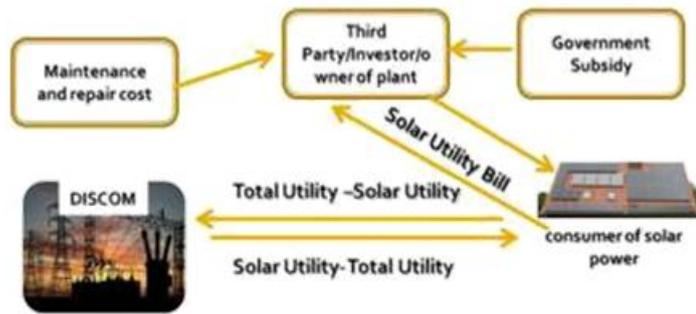
Fig. 3: Layout for the energy transfer processing under RESCO Model.
