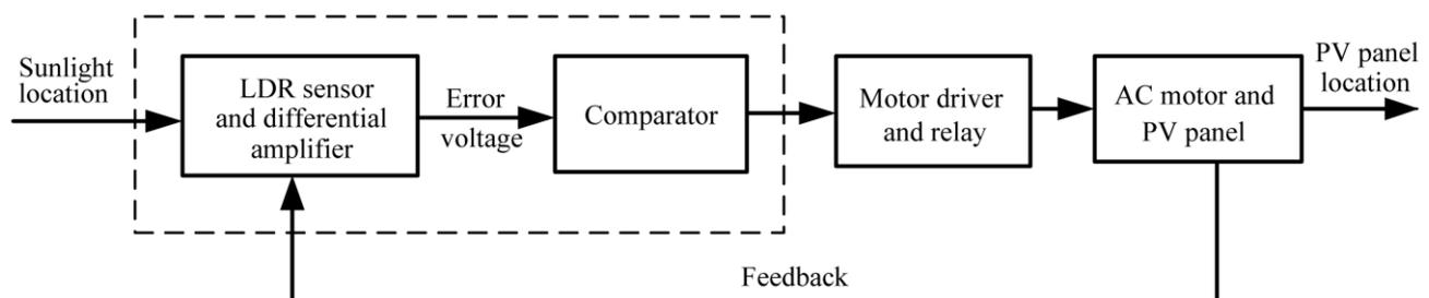
Fig. 6: The operation of the dual axis tracking system totally depends on the LDR
