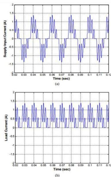
Fig. 8 Passive Wave Shaping method Supply input current and Load Current.
