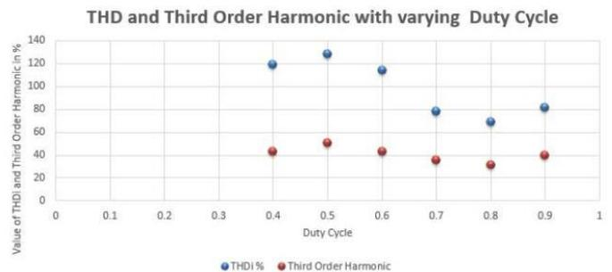
Fig. 6 Variation of THD<sub>i</sub> and 3<sup>rd</sup> order harmonic with respect to duty cycle.
