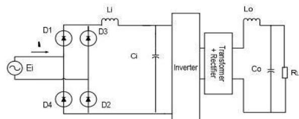
Fig.1 VSF SMR Converter
