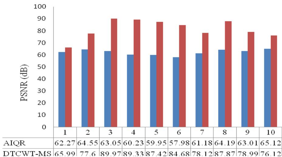
Figure 11. Comparison of PSNR (dB) for the proposed denoising techniques for NOAA images
