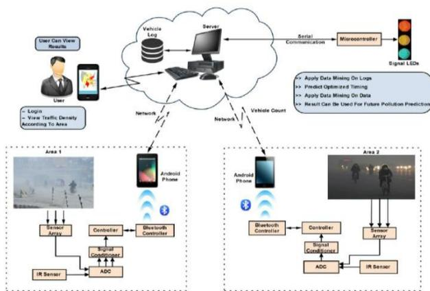
Fig 2.5.1: Architecture of Traffic Congestion & Monitoring System
