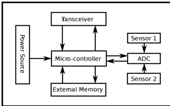
Fig 3.1.1. Architecture of wireless sensor node.
