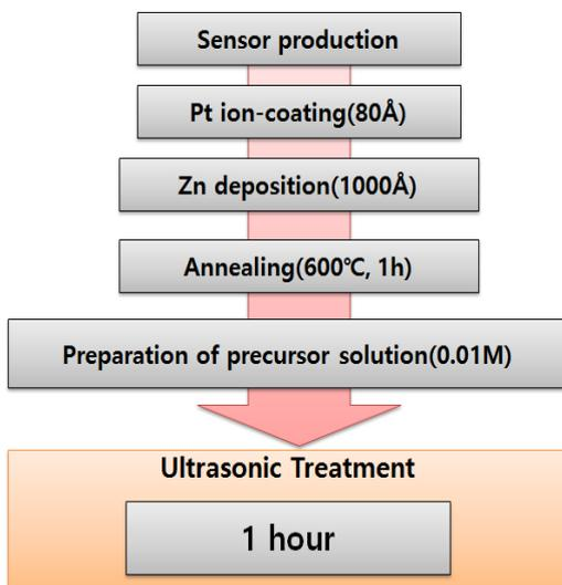
Figure 1. The manufacturing process for the semiconductor type gas sensor
