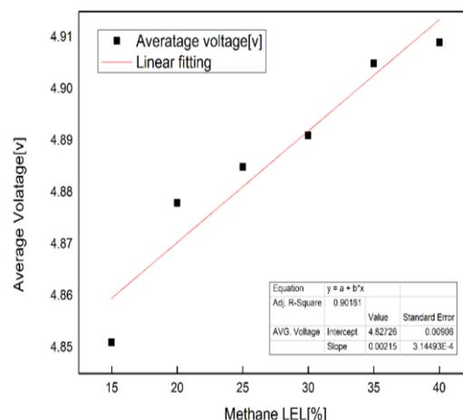
Fig. 6 The response Characteristics of Sensor by Methane Gas Concentration (Average Voltage)
