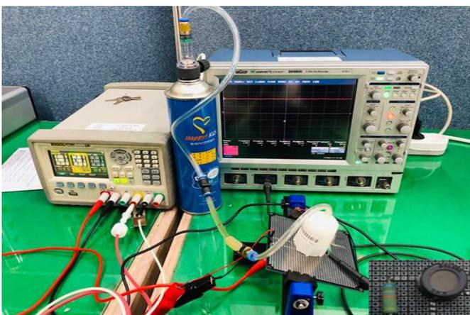
Figure 5. The test equipment of sensors for response characteristic
