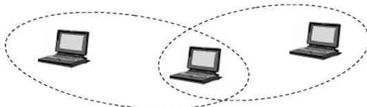
Figure 1.1 AD-HOC network with three nodes
