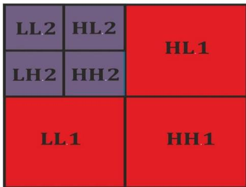
Figure 1: DWT decomposition with two levels.
