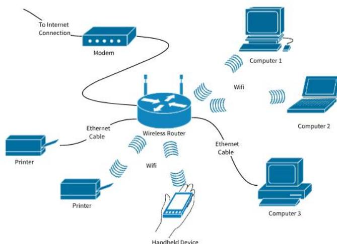
Figure 2: wireless network diagram
