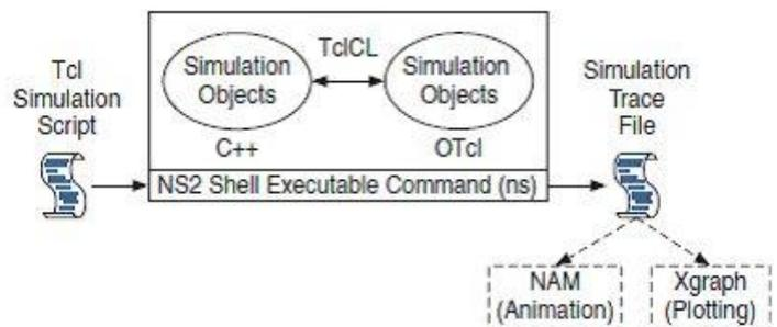
Figure 5: Basic architecture of NS2
