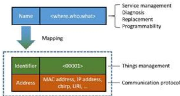
Fig. 5. Naming Mechanism inEdgeOS.
