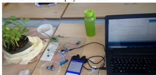
Figure 2:Implementation of smart irrigation system.
