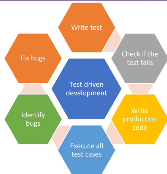
Figure 1 Test driven development stages.
