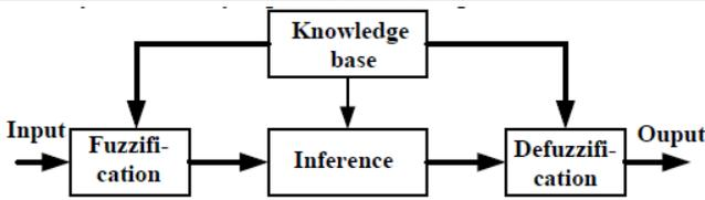
Figure 4.3 Structure of Fuzzy Logic based Decision Making System
