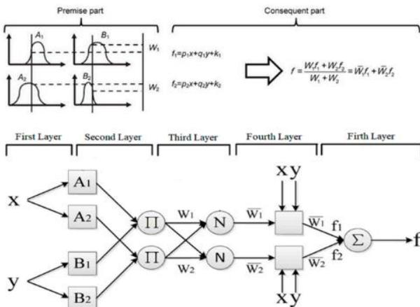
Figure 5.1: ANFIS Structure (Sugeno Model)
