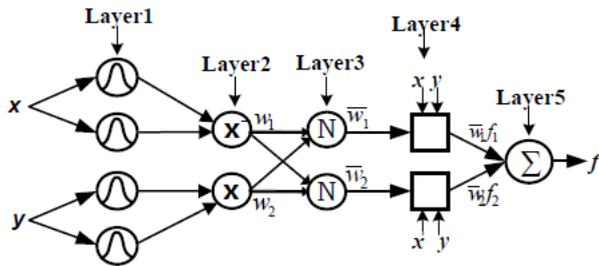
Figure 4.4 Structural Design of Multi-layer-ANFIS
