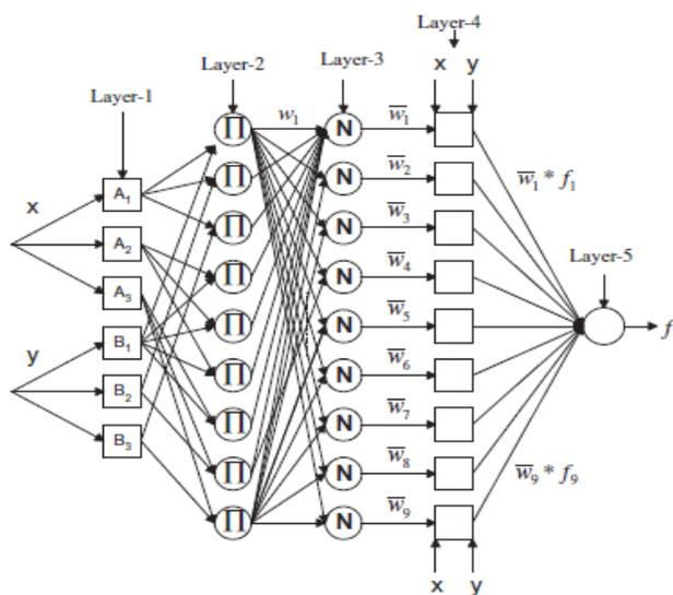
Figure 4.5 Structural Design of Multi-Layer- ANFIS
