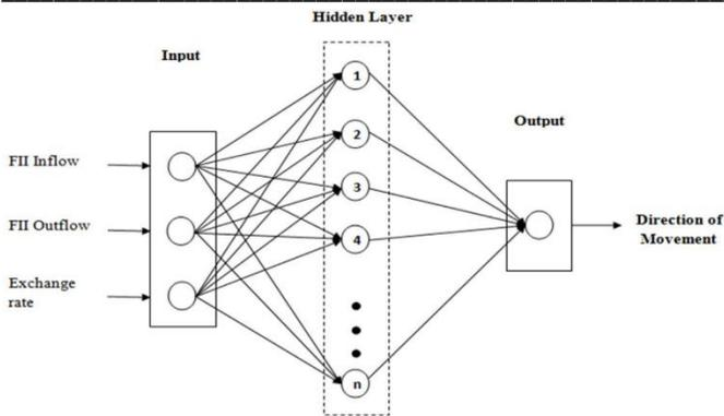
**Figure 4.1 Structural Design of Three Layered Feed forward ANN**
