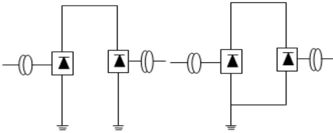
(a) With Crushed Return (b) With Metallic Return
