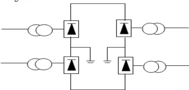
Figure 2 Bipolar HVDC System
