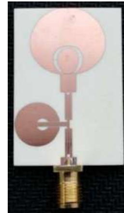
Fig 5. Fabricated prototype of UWB antenna with both arc-shaped slot and multimode resonator filter
