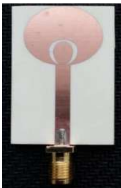
Figure 4. Fabricated prototype of printed planar UWB antenna with an arc-shaped slot
