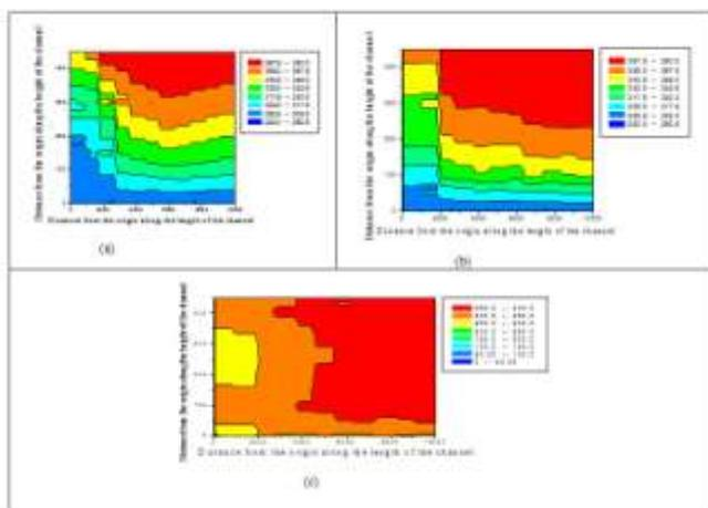
Fig. 13 The coolant fluid temperature distribution of (a) rectangle (b) trapezium (c) triangle cross section over the length at  $(X = Wc/2)$
