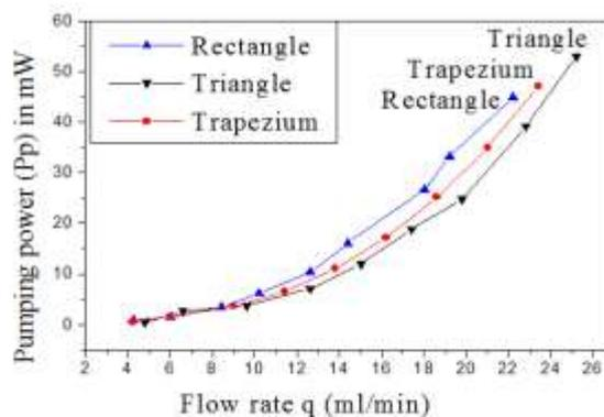
Fig. 5 Variation of pumping power ( $P_p$ ) with flow rate ( $q$ ) in rectangular, trapezium and triangular shaped micro channels
