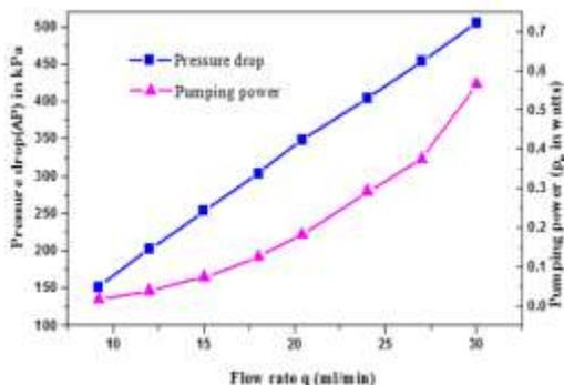
Fig. 15 Pressure drop and pumping power with flow rate for ladder structure triangular shaped micro channel cooling system (LSMCCS)
