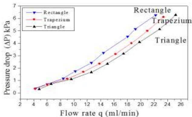
Fig. 4 Variation of pressure drop ( $\Delta P$ ) with flow rate ( $q$ ) in rectangular, trapezium and triangular shaped micro channels
