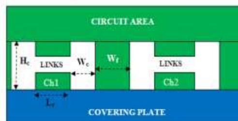
Fig. 1(b). Cross sectional view of the LSMCCS along XX
