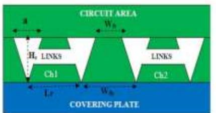
Fig. 3 Cross sectional view of ladder type triangular shaped micro channel cooling system
