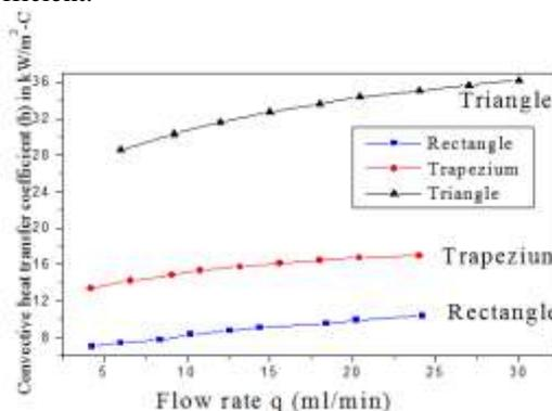
Fig. 11 Variation of convective heat transfer coefficient with flow rate in rectangular, trapezium and triangular shaped micro channels
