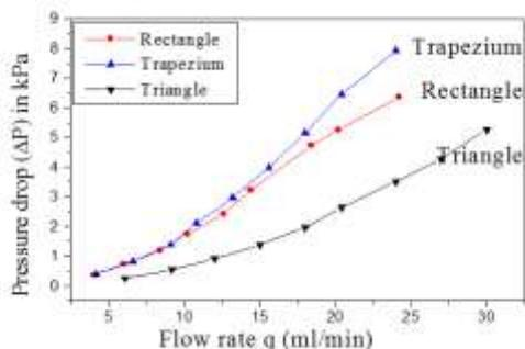
Fig. 9 Variation of pressure drop ( $\Delta P$ ) with flow rate in rectangular, trapezium and triangular shaped micro channels
