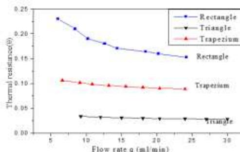
Fig. 12 Variation of thermal resistance with flow rate in rectangular, trapezium and triangular shaped micro channels.
