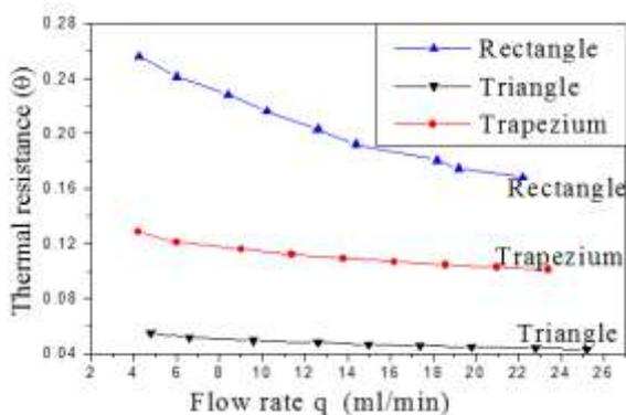
Fig. 7 Variation of thermal resistance (θ) with flow rate (q) in rectangular, trapezium and triangular shaped micro channels
