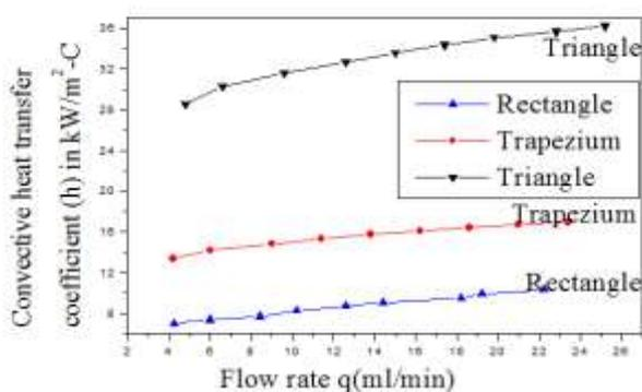
Fig. 6 Variation of convective heat transfer coefficient with flow rate in trapezium and triangular shaped micro channels.
