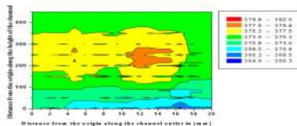
Fig. 20 The coolant fluid temperature distribution in the cross sectional plane at the outlet at (X=0-18000)
