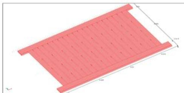
Fig. 13 Created 3D structure of packaged ladder structure triangular shaped micro channel cooling system (Pre-processing)
