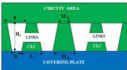
Fig. 2 Cross sectional view of ladder type trapezium shaped micro channel cooling system
