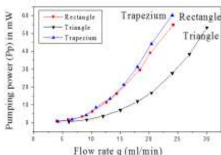
Fig. 10 Variation of pumping power with flow rate (q) in rectangular, trapezium and triangular shaped micro channels.
