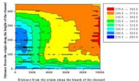
Fig. 18 The coolant fluid temperature distribution in the central vertical plane over the length (y=0-10000) at (X = Wc/2) of the last (Fig. 14) ladder structure micro channel
