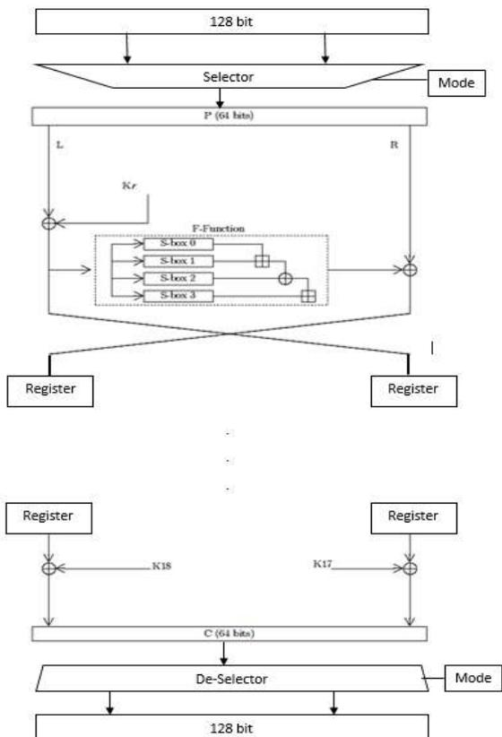
Figure 3: Block Diagram of improved throughput pipelined blowfish Algorithm
