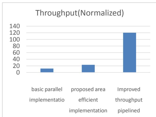
Figure 11: Throughput Comparison among implemented 128bit blowfish algorithms
