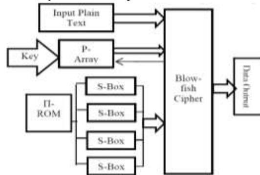
Figure 1: Blowfish Algorithm Design Blocks
