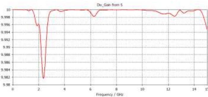
Fig.11. Diversity gain vs frequency for proposed MIMO antenna with orthogonal arrangement
