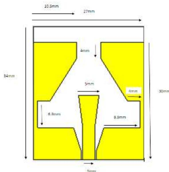
Fig. 1. Proposed UWB antennas system with all dimensions are in millimetres (mm).
