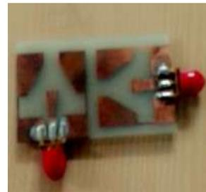
Fig.14. Hardware of Proposed CPW fed UWB-MIMO antenna
