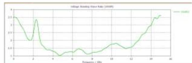
Fig.9. VSWR curve of the proposed MIMO antenna with orthogonal arrangement
