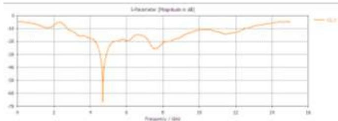
Fig. 7. Return loss curve of UWB-MIMO antenna with orthogonal arrangement (s22)
