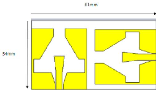
Fig. 2. Proposed UWB-MIMO antennas system with orthogonal placement of antennas
