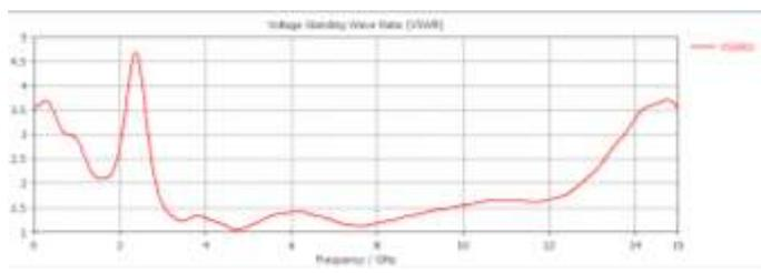
Fig.8. VSWR curve of the proposed single antenna
