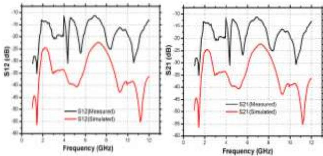
Fig.17. Comparison between simulated and measured result (S12 and S21) of UWB-MIMO antenna with orthogonal arrangement
