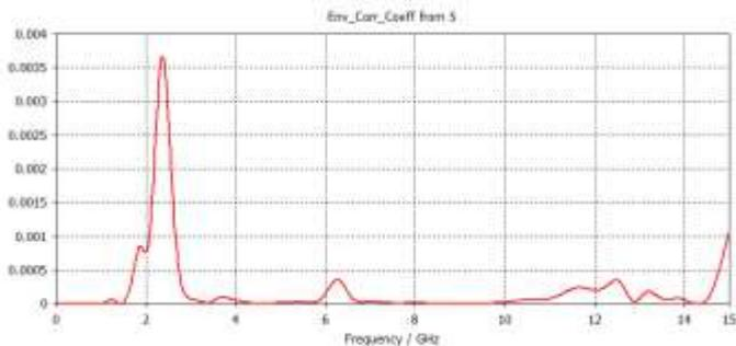
Fig.10. ECC vs frequency for proposed MIMO antenna with orthogonal arrangement
