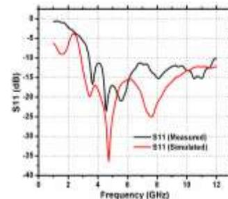
Fig.15. Comparison between simulated and measured result (S11) of primitive antenna
