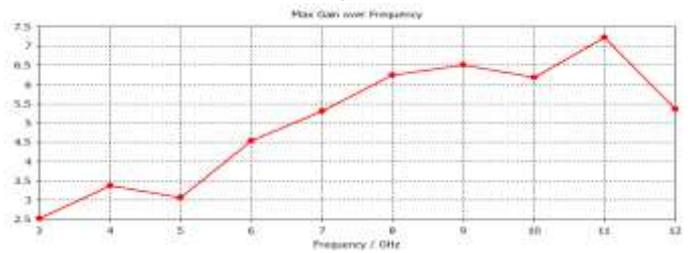
Fig.13. Maximum gain vs frequency for proposed MIMO antenna with orthogonal arrangement
