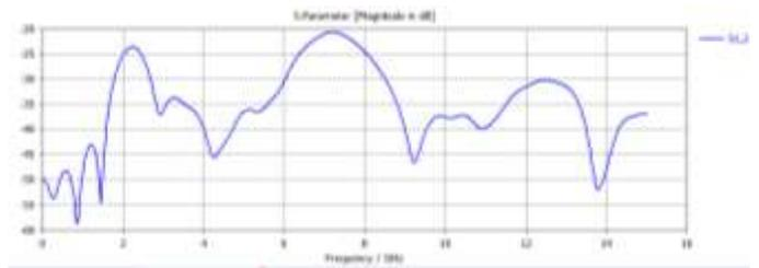
Fig. 5. Return loss curve of UWB-MIMO antenna with orthogonal arrangement (s12)
