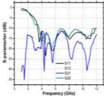
Fig.18. Measured isolation curve of the proposed UWB-MIMO antenna with orthogonal arrangement
