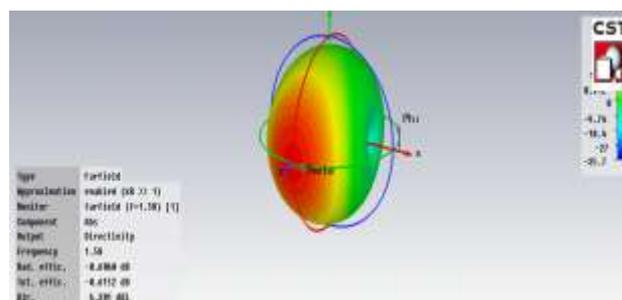
Fig. 7. This is the simulated result of design in figure 5, showing radiation pattern with efficiency and directivity.
