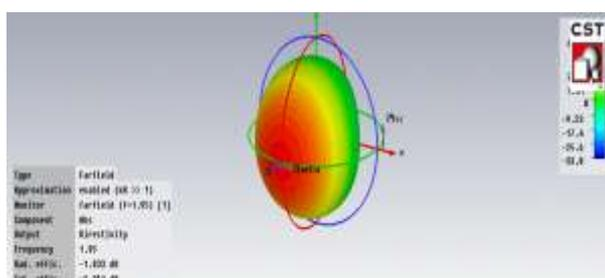
Fig. 3. Simulation result shows directivity, efficiency and radiation pattern.
