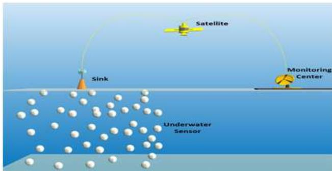
Fig 3.1.1: Under water sensor
