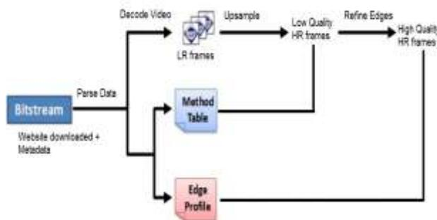
Figure 6. Upsampling at Mobile Client
