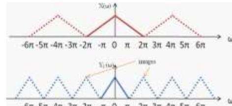
Figure 3. Frequency domain representation before and after interpolation
