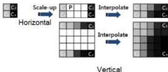
Figure 5. Upscaling in horizontal and vertical direction
