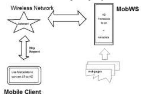
Figure 1. System Architecture for MobWS
