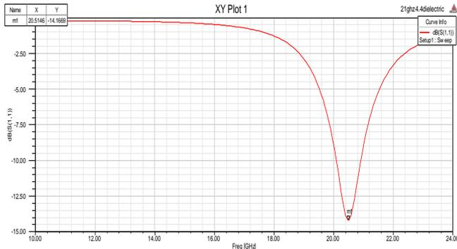
Figure2.Simulation of Return Loss S11 of Microstrip Patch Antenna without Metamaterial.
