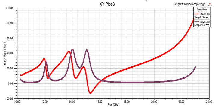
Figure7. Input impedance of proposed metamaterial SSR structure.
