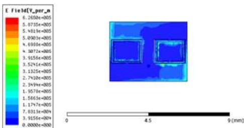
a).E-Field current distribution at 12.12Ghz b).E-Field current distribution at 14.23Ghz
