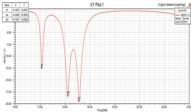
Figure4. Return loss of proposed metamaterial SSR structure
