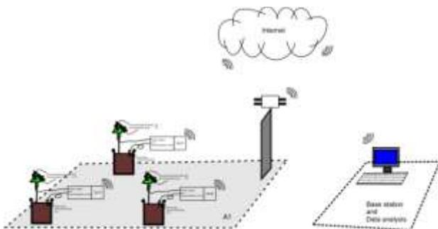
Figure 2. (Network star topology architecture) Distribution of the modules for a surface  $A_1$ .
