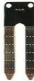
Figure 3. Conductive plate transducer
