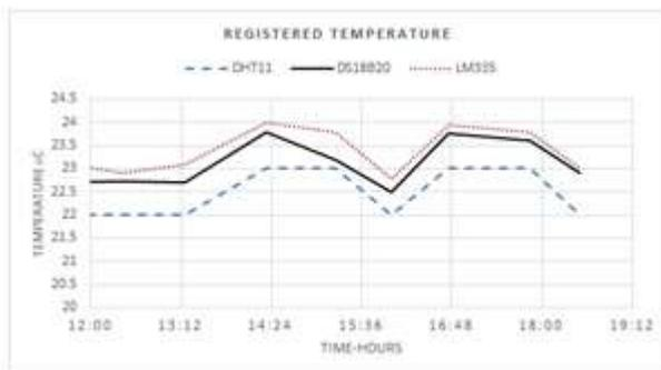
Figure 5. Temperature graph recorded by the different sensors. X axis presents the temperature and the Y axis the time range in hours
