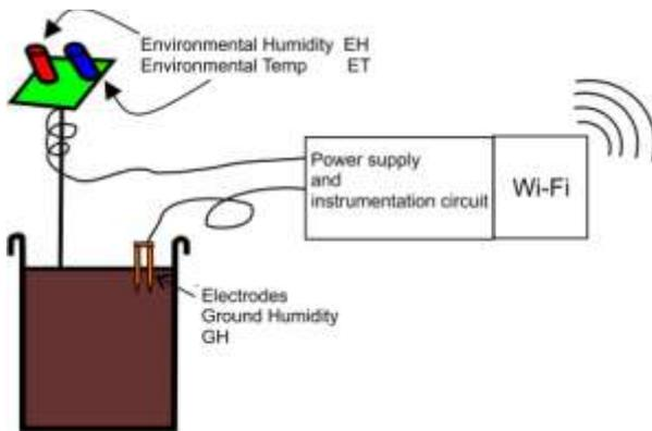
Figure 1. Individual module for the registry of the environmental physical
