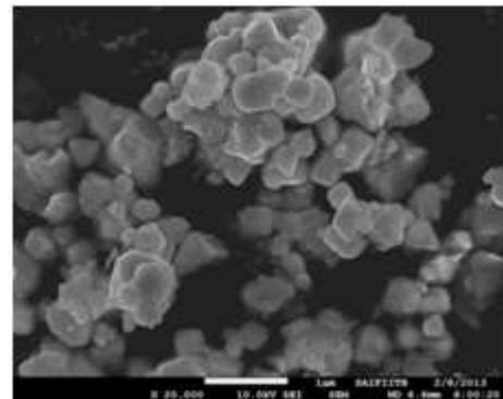
**Figure 5: SEM micrograph of PLZT (10/52/48) powder calcined at 850 °C for 3 hrs.**
