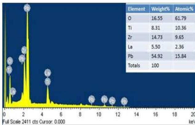
Figure 7: EDAX measurements for PLZT (10/52/48) powder.
