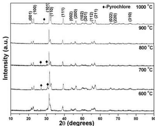
**Figure 4 XRD patterns of PZT powders calcined at different temperatures.**
