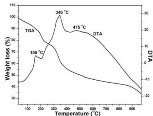
Figure 2: The thermogravimetry (TG) and differential thermal analysis (DTA) of dried gel in helium environment.
