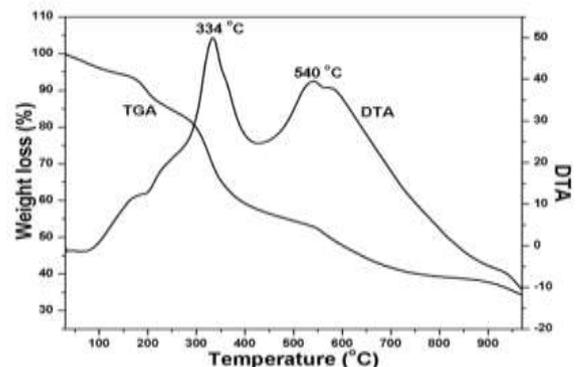
Figure 1: TGA/DTA curve for the PZT powders synthesized by sol-gel route
