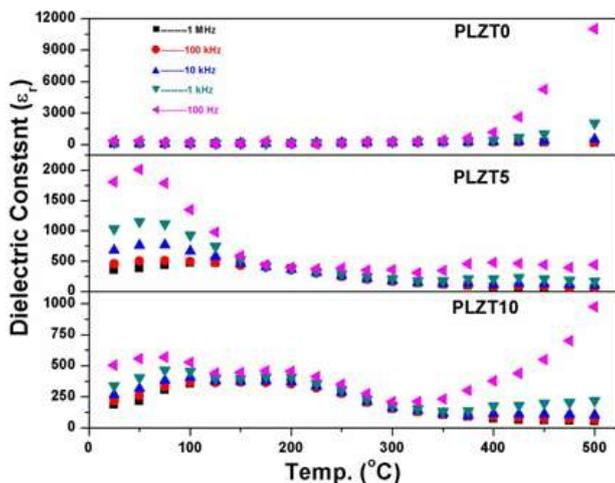
Figure 8 Dielectric permittivity vs temperature for compositions 0/52/48, 5/52/48 and 10/52/48 at various frequencies.
