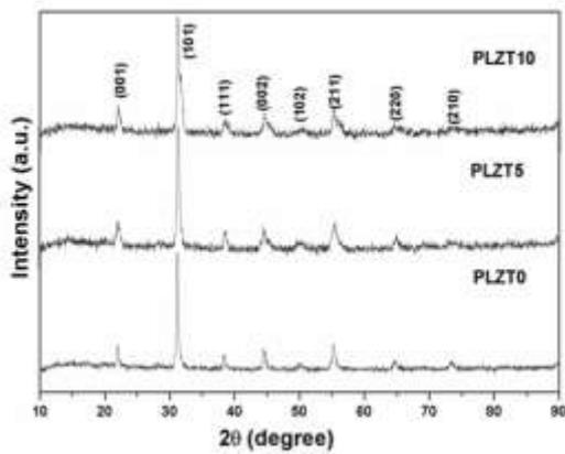
**Figure 3 Room temperature XRD patterns of PZT ceramics with various % of La content.**
