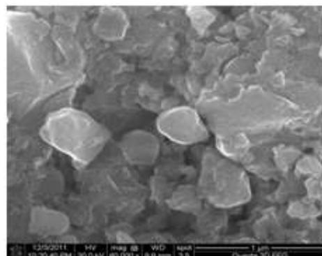
**Figure 6: pellet after sintering at 875 °C for 4 hrs**
