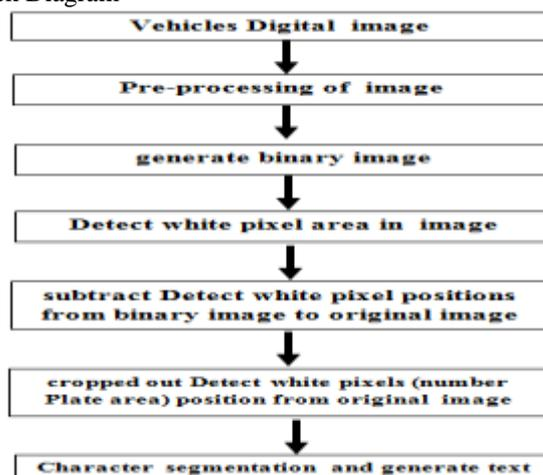
Fig.2. Framework of the proposed number plate detection approach.
